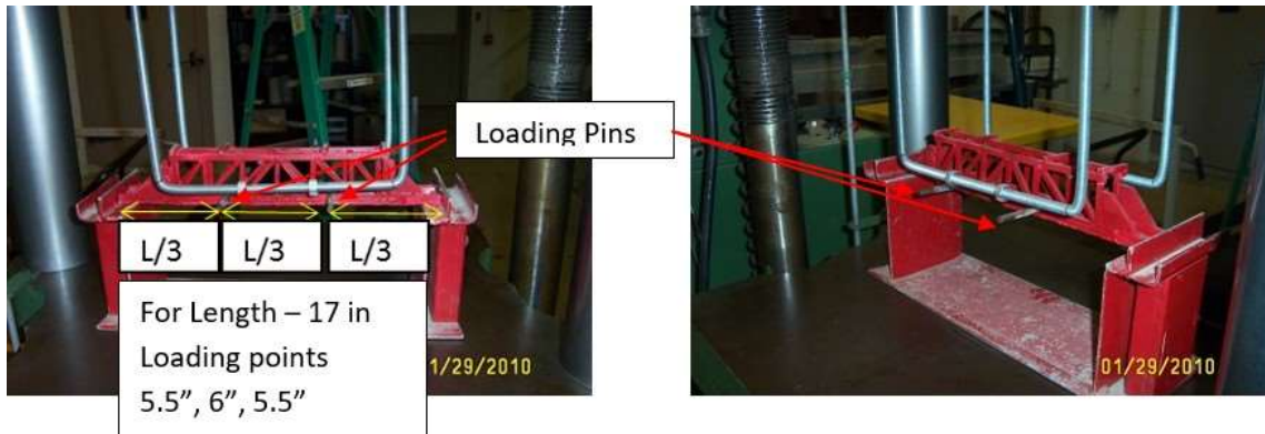
Figure 2. Typical bridge testing setup
